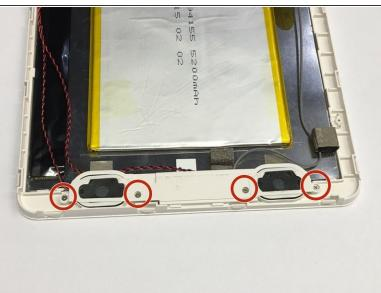
Using a J0 phillips head bit, remove the four 1mm screws from the speaker cover. Remove the cover and all four screws.
