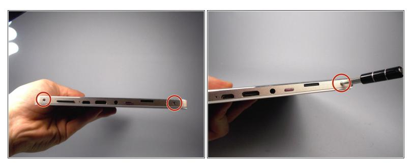
Remove the two screws from the top of the tablet as shown in the figure using a J0 philips head bit.
