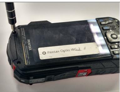
Remove all four 1 mm JIS #00 screws from the back of the camera.
