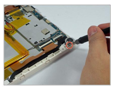
Using a J0 phillips head bit, remove the single 1 mm screw from the rear facing lens cover.
