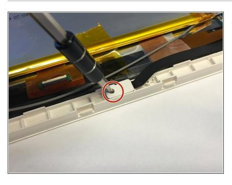
Using a J0 phillips head bit, remove the single 1mm screw from the front facing camera lens cover.
