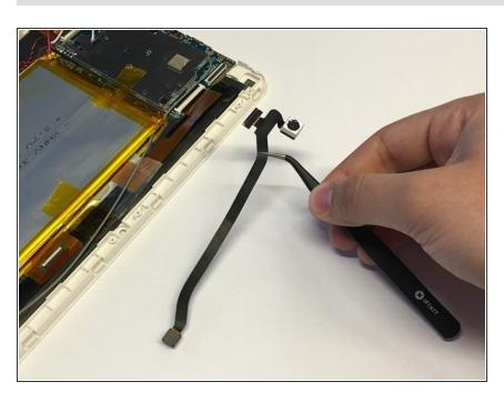
Remove the camera strip from the device.
