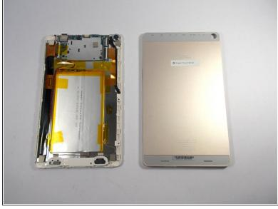
• Using your hands and the separating tool, remove the back cover from the device.
