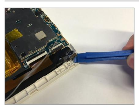
Using a plastic opening tool, pry the rear facing camera out of its housing.
