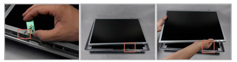
Be careful of the wires attaching the power button and the control buttons. Show extreme caution to ensure the button is not damaged.
