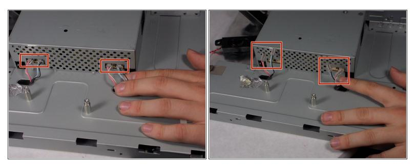
• Remove the 4 connectors from the left side of the monitor on the back.
