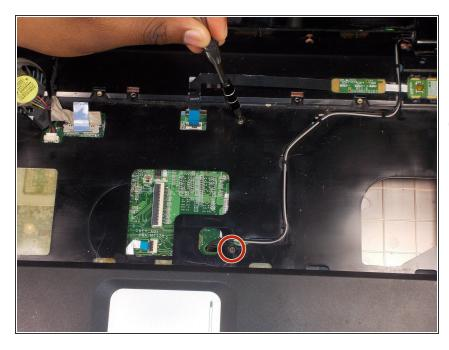
Remove two 5.5mm screws holding the chassis top down from underneath the keyboard.
