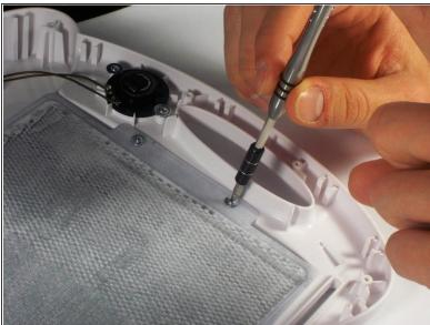
Remove the four 5mm PH 0 Phillips screws with 7mm heads holding the screen to the front of the case.
