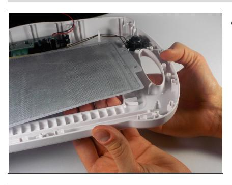
Gently push the edges of the screen to remove it from the front case.
