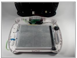
Remove all eleven 9mm PH 2 Phillips screws securing the back of the case.
