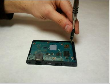
Remove the last 6mm Phillips #0 screw from the motherboard.
