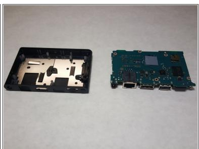
Use a plastic opening tool to pry up gently on the motherboard, and remove it.
