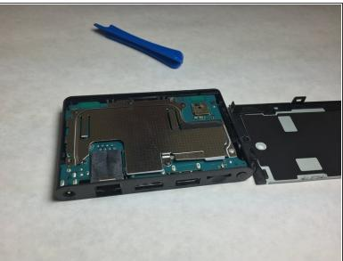
Use the plastic spudger to pry up the bottom piece of the case to release the clips.
