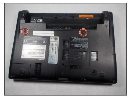
Locate the two 1.2mm philips #000 screws holding the bottom plate onto the laptop.
