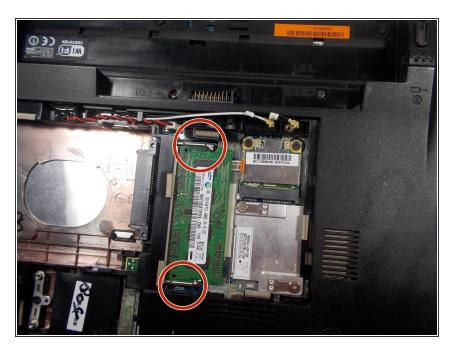
Locate the two small prongs on each side of the RAM.
