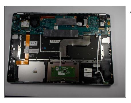
Lift up and remove the Lithium-Polymer Battery.
