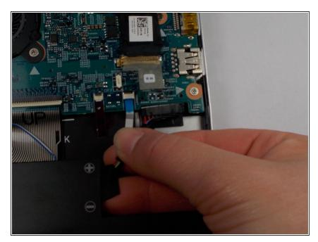
Disconnect the ribbon cables from the motherboard.
