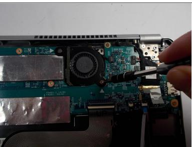
Remove the two 2.5 mm screws using a J000 Phillips Head Screwdriver.
