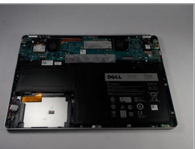
Pry open the back cover using a spudger and slide it along the under the cover.
