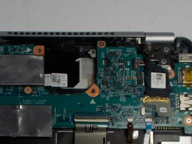
Pull up on the wire and remove the Cooling Fan.
