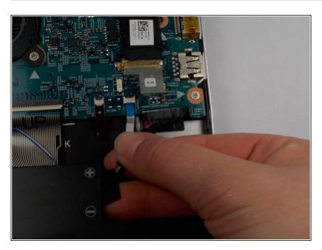
Disconnect the ribbon cables from the motherboard.
