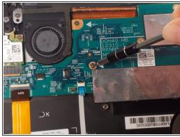
Remove the eight 2.5 mm screws using a J000 Phillips Head Screwdriver.
