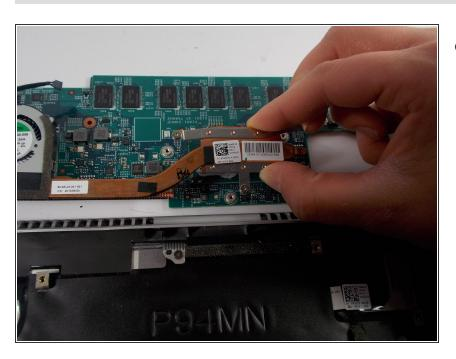
Remove the Thermal-Cooling
