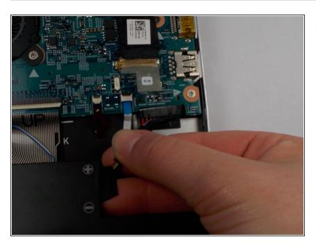
Disconnect the ribbon cables from the motherboard.
