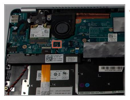
Disconnect wires from Motherboard by gently pulling up.
