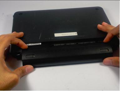
With the left switch still pushed inward, pull the battery towards you to remove it from the computer.
