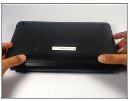
With the bottom of the HP Mini facing up, slide both switches inward towards each other.
