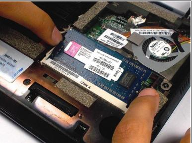
Push the two white holders holding the RAM outward until it points upwards at about a 45 degree angle.
