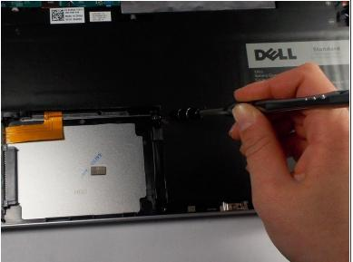
Remove the two 2.5 mm screws holding the battery in place using the J000 Phillips Head Screwdriver.
