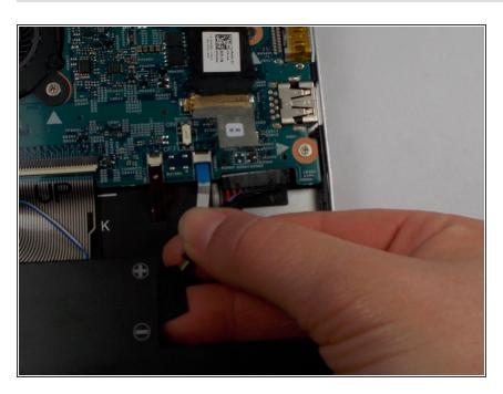
Disconnect the ribbon cables from the motherboard.
