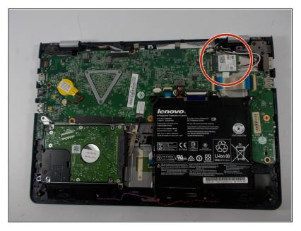
• Locate the network card on the top right of the computer.
