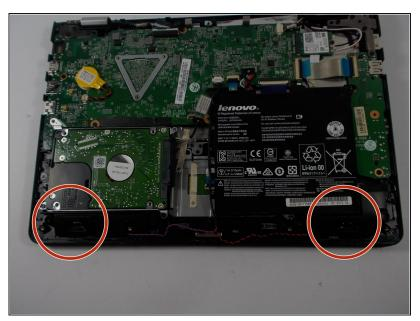
• Locate the speakers at the bottom left and right corners of the computer.
