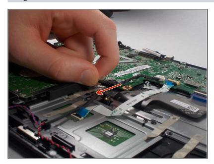
• Pull the connector out of its port on the motherboard.
