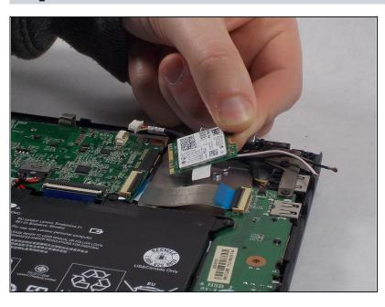
Slide the network card out to the right to remove it from the motherboard.
