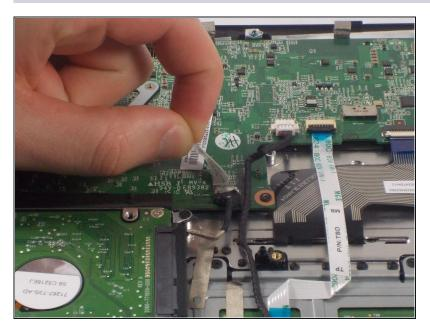
Lift off the strip of tape securing the wire down to the computer.
