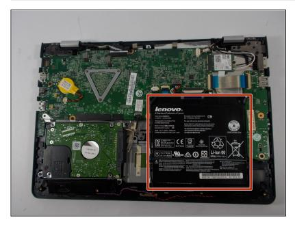
Locate the black battery on the bottom right of the computer.
