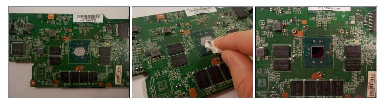
• Wipe the residual paste off of the processor on the motherboard with a clean cloth.
