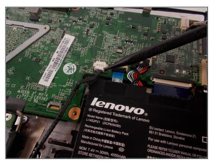
Using the spudger, pull the wire down and away from the motherboard to disconnect it.
