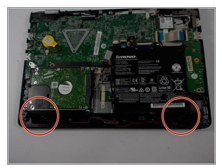
Locate the speakers at the bottom left and right corners of the computer.
