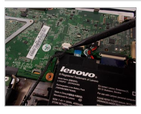
Using the spudger, pull the wire down and away from the motherboard to disconnect it. To reassemble your device, follow these instructions in reverse order.
