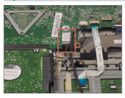
Follow the wire out from the right side of the hard drive to locate where the hard drive connects to the motherboard.
