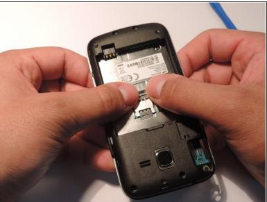
Unscrew the 1.2mm Phillip screw that connects the motherboard to the rest of the phone. Then by using your thumbs pop the inners of the phone out. Also use same J00 Phillips head bit from prior steps.
