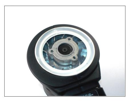
Once the sander pad is removed and the sander is exposed locate the white plastic like circular piece
