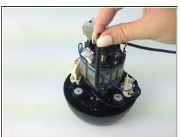
• Remove the cooling pipe from the top inside of the blender base and replace it.
