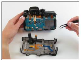
Use tweezers to pull the two ribbon cables horizontally out of their clips.
