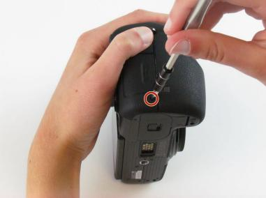
Use the Phillips #00 screwdriver to remove the two 5.5 mm screws from the right side of the camera above the SD card port.
