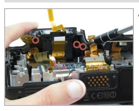
Use the Phillips #00 screwdriver to remove the three black 3.8 mm screws below the viewfinder.
