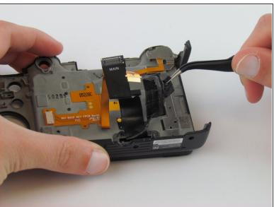
Use tweezers to remove the glued rubber piece.
