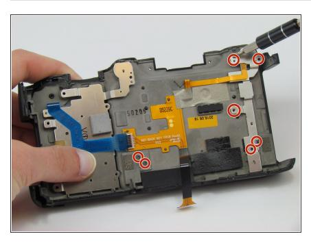
Use the Phillips #00 screwdriver to remove the seven screws (three silver 3.5 mm screws and four black 2.7 mm screws).
