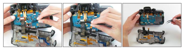
• Use <u>tweezers</u> to pull the two ribbon cables horizontally out of their clips.
