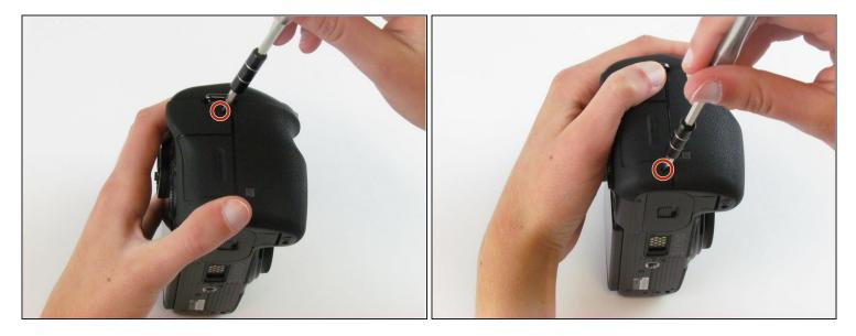
• Use the Phillips #00 screwdriver to remove the two 5.5 mm screws from the right side of the camera above the SD card port.
