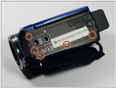
Remove the five 30mm Phillips #0 screws on the bottom of the camera.
