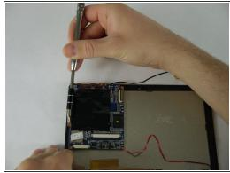
Using a PH0 screw bit unscrew the three 3mm screws securing the motherboard to the back panel.
