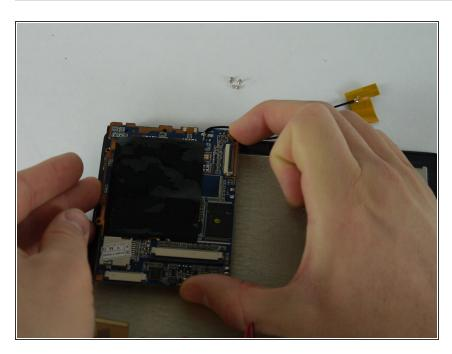
Carefully lift up on the motherboard from its housing.
