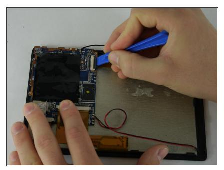
Using a plastic opening tool lift up the flap on the ribbon cable receptacle.
