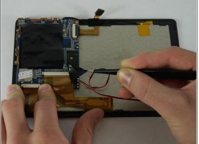
• Using a pair of tweezers begin to peel the tape covering the ribbon cable on the motherboard.
