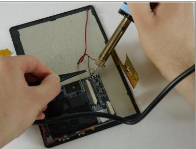
Desolder the wires that connect the backlight to the motherboard.
