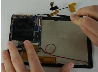
Using a pair of tweezers remove the camera assembly from its housing and its receptacles.
