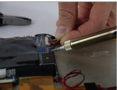
Desolder the wires that connect the battery to the motherboard.
