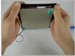
Gently pry the brackets holding the touch sensor to the LCD Screen
