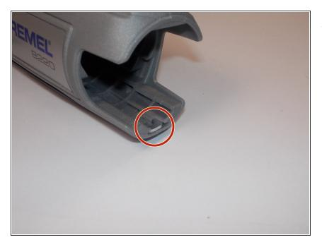
Remove the metal clasp from the battery well. This piece helps hold the plastic shell of the device together. Pry it out by gently applying some force with a screwdriver.
