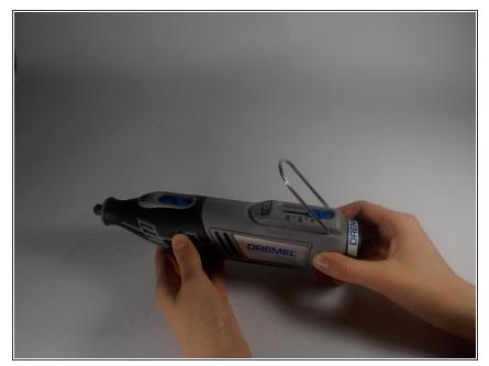
Locate the battery at the back of your Dremel. Firmly grasp the battery on both sides and pull. It should easily come out of the battery well.
