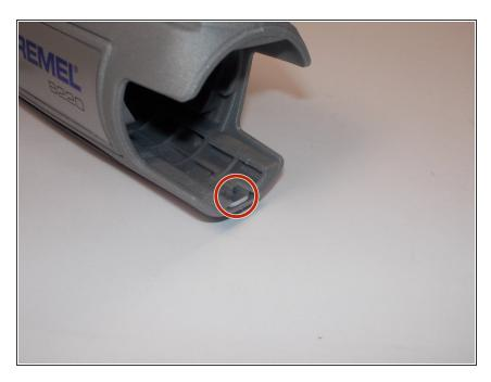
Remove the metal clasp from the battery well. This piece helps hold the plastic shell of the device together. Pry it out by gently applying some force with a spudger.
