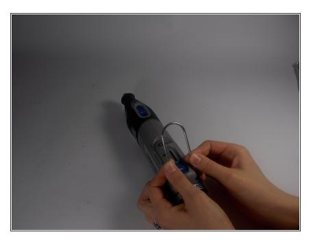
Remove the ring located around the speed selector switch by pulling apart on either side. (This should require very minimal force.)
