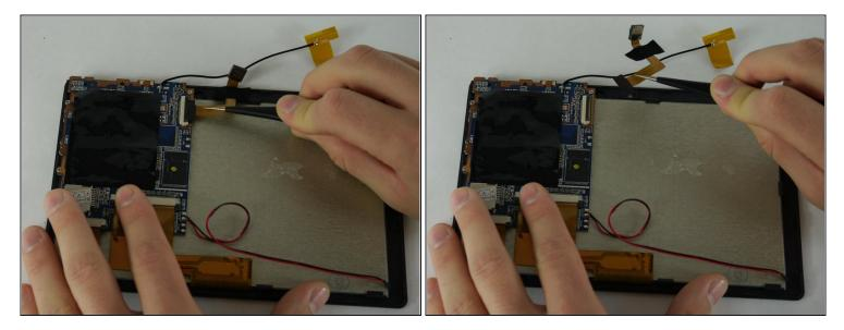
• Using a pair of tweezers remove the camera assembly from its housing and its receptacles.
