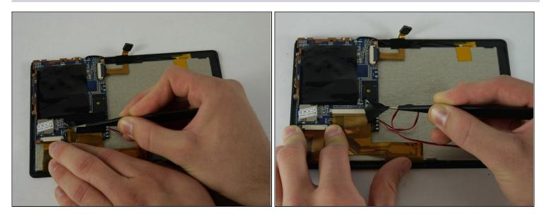
• Using a pair of <u>tweezers</u> begin to peel the tape covering the ribbon cable on the motherboard.
