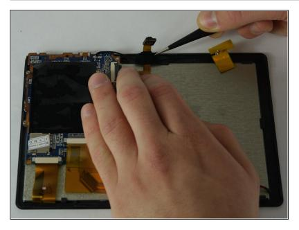
• Using a pair of tweezers remove the tape securing the cameras to the back panel.
