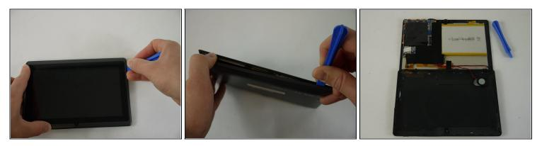
• Using a plastic opening tool, carefully pry the device apart. Make your way around the entire perimeter of the device and carefully place the two panels next to each other.
