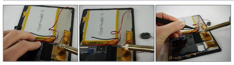
• <u>Desolder</u> the speaker wires from the motherboard.
