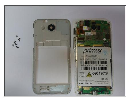
Remove the screws and exerting a little pressure remove the plastic cover.
