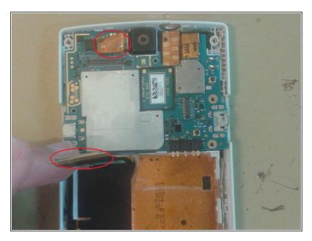
To remove the battery, remove the two buses pointed out in red.
