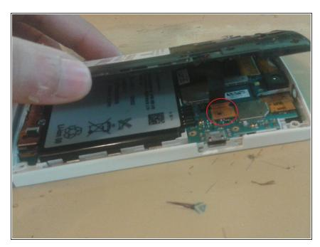
Then, detach the first bus (indicated with the red circle) to fully detach the case.
