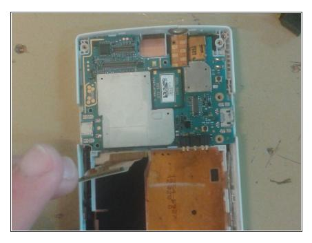
After removing the buses, we can remove the camera and the motherboard. Proceed to remove the motherboard.
