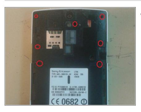
Remove the screws in the indicated areas (Red Markings) with a screwdriver.
