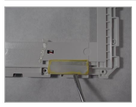
Now peel off the final screen, protecting the speaker.
