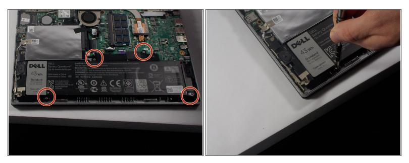
Locate the battery at the bottom of the computer and remove the four 3mm screws with a Phillips #0 head that hold the battery down.
