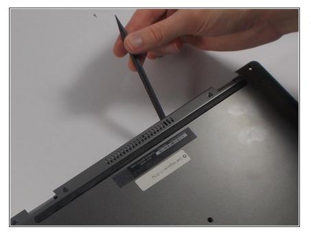
Gently use a spudger to pull the cover away from the rest of the laptop. The cover will come off after you use the tool on two or three sides.
