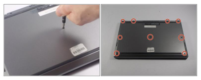
• Remove all nine 5mm Phillips head screws from the back cover using #0 Phillips head.
