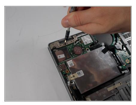
Unscrew the brackets in the top right and top left of the laptop. Unscrew the two 1mm screw from both of the
