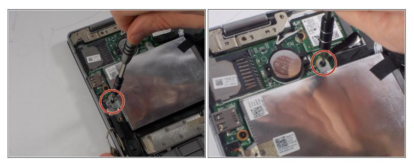
• Remove all three 2mm screws holding down the Solid State Drive by using a #0 Phillips head.
