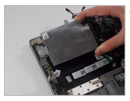
• Remove the Solid State Drive by simply lifting it away from the laptop.
