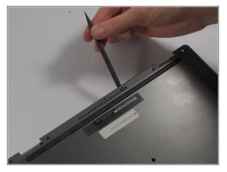
Gently use a spudger to pull the cover away from the rest of the laptop. The cover will come off after you use the tool on two or three sides.
