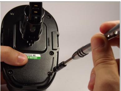
Remove the six 19 mm, Torx Security 15 screws from the top of the battery.
