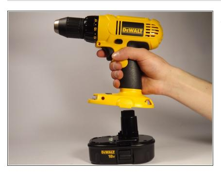
Remove battery from drill.
