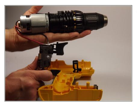
• Lift drill mechanism from the drill assembly.
