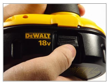
Compress the buttons on either side of the battery and lift the drill away from battery.
