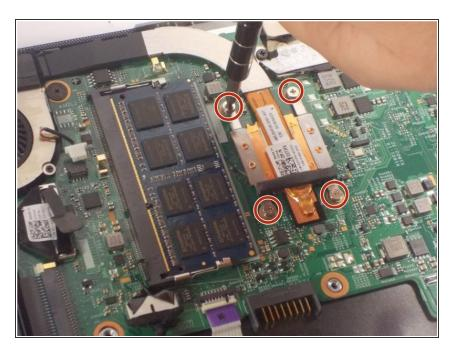
Remove the four 3mm screws using a Phillips #0 head.
