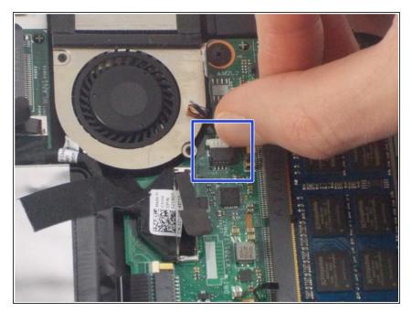
Using your fingernail, unplug the white power cable connector to the right of the cooling fan by pushing it away from the port.
