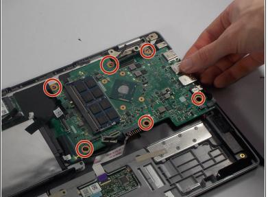
Unscrew six 1mm screws holding down the motherboard using a #0 Phillips head.
