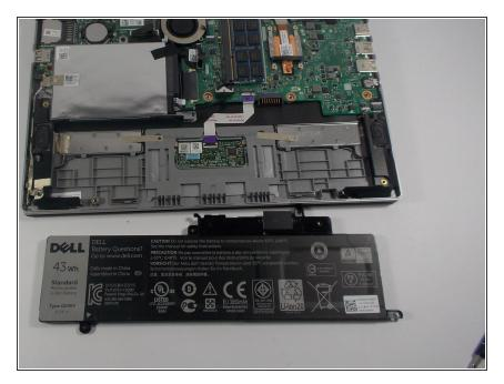
Remove the battery from the computer system by gently lifting it from the side.
