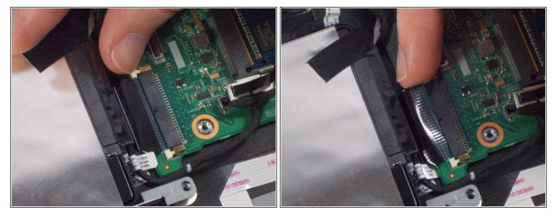
Slide the ZIF cord connecting to the Solid State Drive towards itself to detach it from the motherboard.
