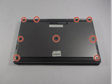
Remove all nine 5mm Phillips head screws from the back cover using #0 Phillips head.
