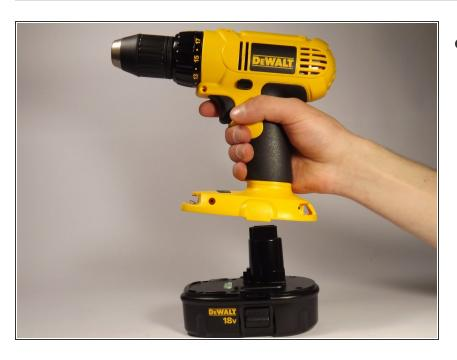
Remove battery from drill.
