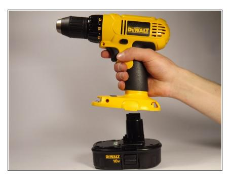
• Remove battery from drill.
