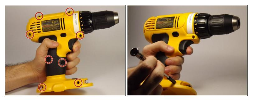
Remove the eight 16 mm, Torx Security #15 screws.
