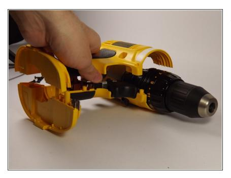
• Lay the drill on its side and gently lift the top half off it.
