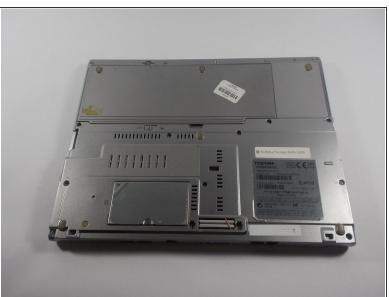
Flip the laptop over. Keep the front end facing away from you, so the battery appears at the top.
