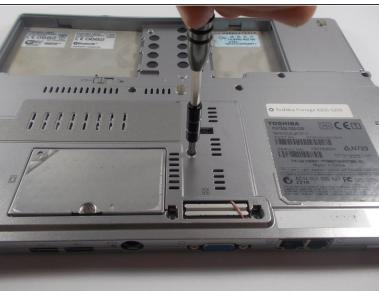
Remove the 4mm Phillips head screw in the middle of the laptop with a Phillips head #00 screwdriver.
