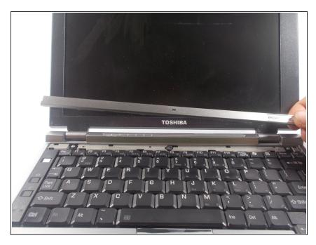
Lift up and remove the plastic casing.
