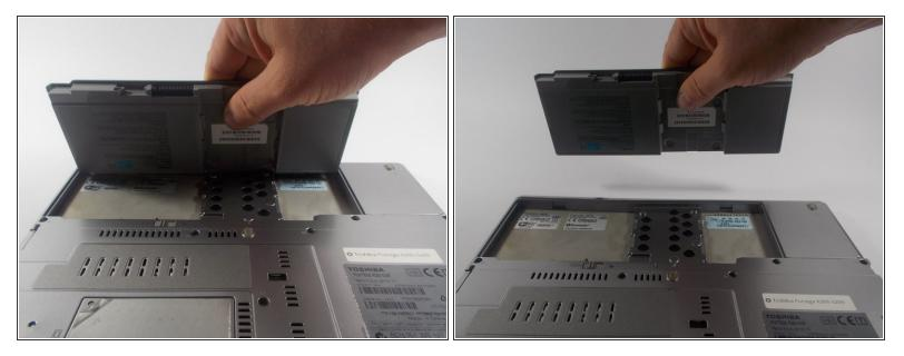
Remove battery by lifting upward.
