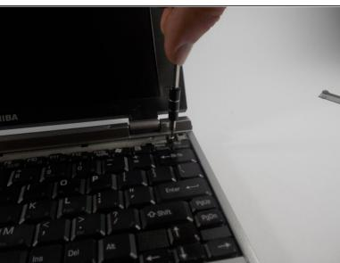
Remove the 4mm Phillips head screws at the top of the keyboard at both ends, using the Phillips head #00 screwdriver.
