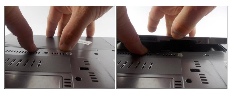
While holding the locking mechanism to the right, insert your finger into the tab and lift up.
