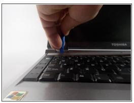
Remove the plastic casing above the keyboard with the plastic opening tool. Start at the edges of the plastic casing and move toward the middle.
