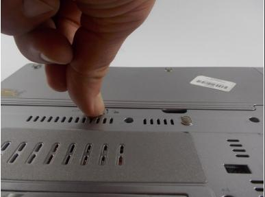
Slide the locking mechanism to the right and hold.
