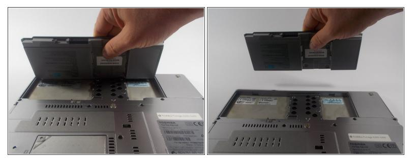
Remove battery by lifting upward.
