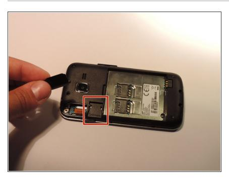
After following the steps for battery replacement, the SD memory card is going to be able slide right out of this slot for replacement.
