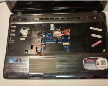
Check if the touch pad cable is plugged into the ZIF connector on the motherboard.
