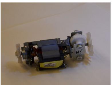
Once disconnected, the motor will slide out easily.
