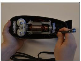
Remove the four 8.6 mm Philips #2 screws securing the motor mount and place them aside.
