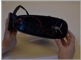
Remove the seven 1.3 mm Philips #2 screws that attach the motor casing to the mixer handle and set them aside.
