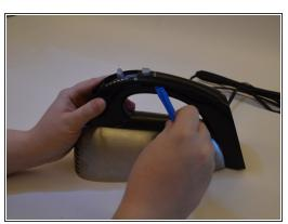
Use a plastic opening tool to take off the handle's cap by loosening both ends and then sliding the tool to the middle of the handle.
