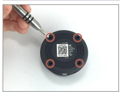
Remove the four 6 mm screws from the back panel with the J000 Phillips head screwdriver.
