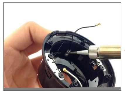
Using a soldering iron, melt away the base of the Wi-Fi cable until it can be removed. <u>Use this guild for assistance</u> with soldering.
