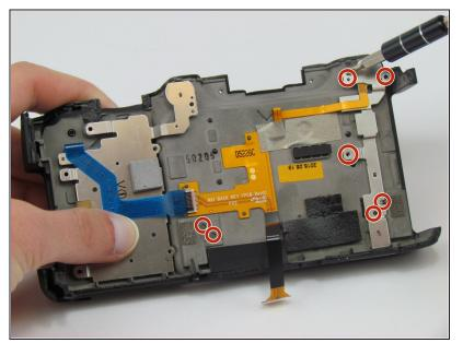
Use the Phillips #00 screwdriver to remove the seven screws (three silver 3.5 mm screws and four black 2.7 mm screws).
