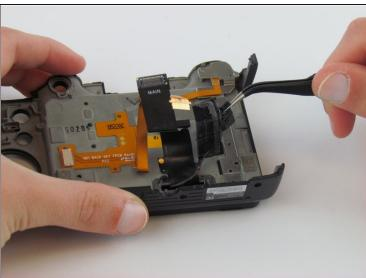
• Use <u>tweezers</u> to remove the glued rubber piece.
