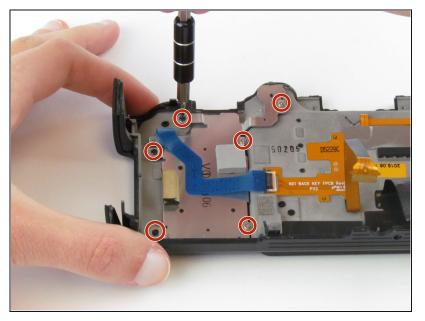
Use the Phillips #00 screwdriver to remove the six screws (three silver 3.5 mm screws and three black 4.2 mm screws).
