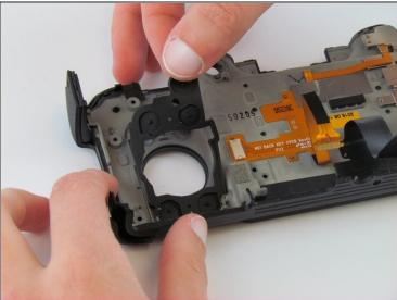
• Use your fingers to remove the metal piece with the blue ribbon cable and the rubber buttons lying underneath.
