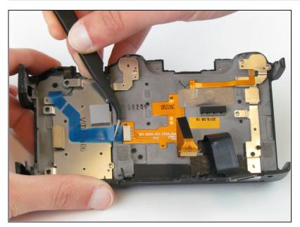
Use the <u>tweezers</u> to pull the blue ribbon cable horizontally out of its clip.
