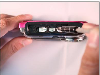
Apply pressure and turn counterclockwise to remove the indicated 2.5 mm screw.
