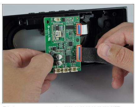
Gently pull out the two ribbon connectors to disconnect the motherboard from the case.
