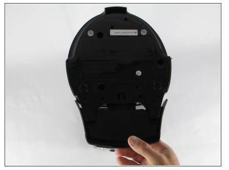
Carefully slide off the bottom drip tray by sliding it out away from the Brew Station.
