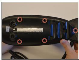
Flip the handle on its side. Remove five 3.8 mm Philips #2 screws shown and set aside them aside.
